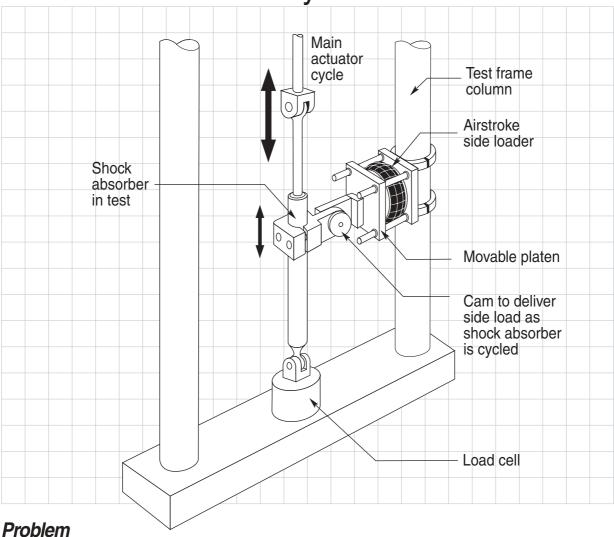
System needed to simulate side load pressure on shock absorber units to produce wear on seals and rod during cyclic testing. Current systems utilize weights, pulleys and cables to produce the effect.
